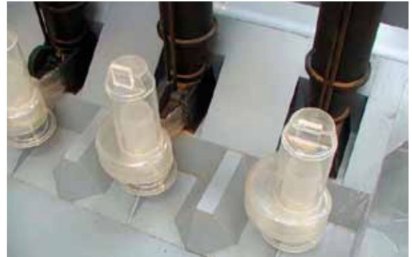
Centrifugal pump sump design verified by a scale model test.
