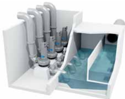
Rectangular sump with high side-entry inlet shown with dry-installed pumps.
