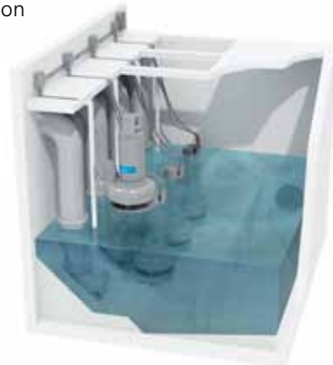
Rectangular sump with low side-entry inlet shown with submersible pumps.
